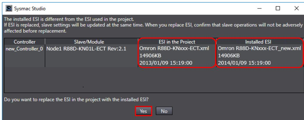
**9.2.2. Checking the EtherCAT Network Configuration**
