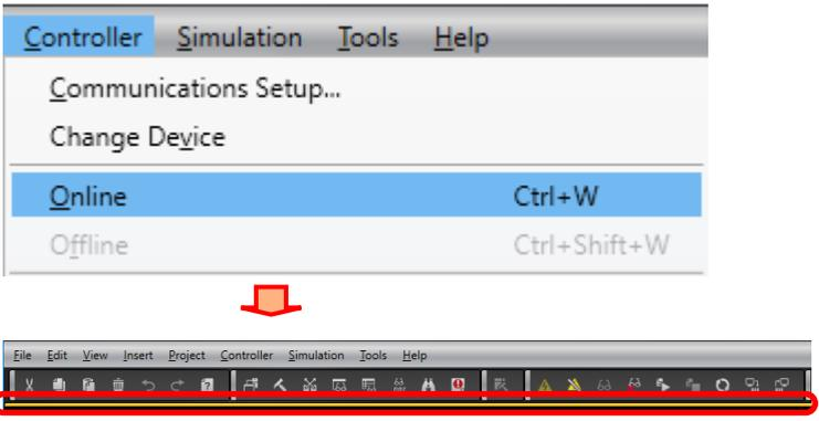
When an online connection is established, a yellow line is displayed under the toolbar.
