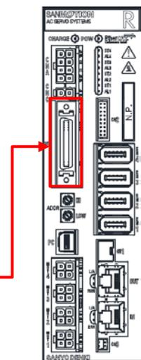
The closing brace bracket to the right of the table above indicates the bits that are assigned to the general I/O connector shown on the right (boxed in red).
